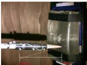
The target consisted of a block of PermaGel™, a clear synthetic muscle simulant. A load cell inserted into the spear shafts captured force profiles (Newtons) and were translated into data by Imatek Impact Analysis software. Each spear thrust was filmed using Phantom V7 high speed video camera (1000 fps). Videos were analysed for impact velocity. Depth of penetration was also measured.
